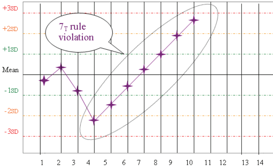
Fig. 11. Rule 7T - reject when seven control measurements trend in the same direction, either higher or lower.
